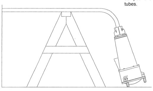
4. Place the coupler as close to vertical as possible, this will ensure the compound fully fills the phase insulator tubes.
