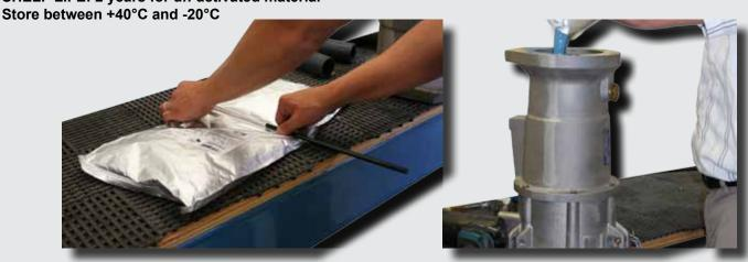
1. After terminating the cable and reassembling the coupler arrange the coupler so as to expose the rear body entrance.
