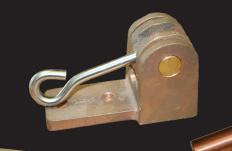
Our cast bronze alloy cam clamps are universally compatible with other manufacturers' products. The clamps are ideal for high voltage or unusual uses where cable couplers are not appropriate. There are two parts required to make a cam clamp assembly: the cam clamp bushing, which is soldered to a portable cable conductor; and the cam clamp, which is bolted to a bus bar or terminal pad. The bushing is inserted and clamped into the cam clamp.
