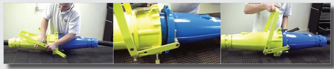
The closing tool allows for quick and easy connection and disconnection by one person.
