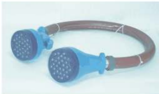
Locomotive-to-Locomotive or Car-to-Car Jumper equipped with Safety Decoupler
