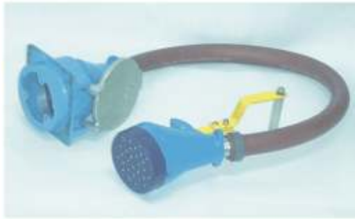
Locomotive-to-Locomotive or Car-to-Car Jumper equipped with Disconnect Handle shown coupled with Plug
